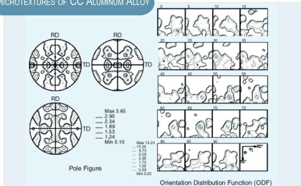
Orientation Distribution Function (ODF) result and pole figure for a thermomechanically processed continuous cast aluminum alloy.
